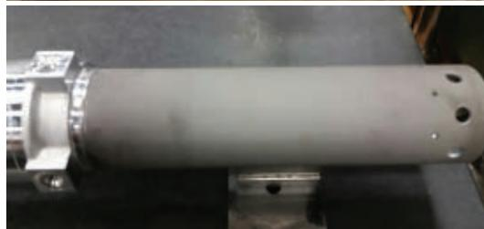
High-velocity oxygen fuel (HVOF) spraying of coatings was developed to apply ultrahard, corrosion-resistant coatings to steel substrates. The hardness and thickness of the coatings makes them difficult to grind. Photos courtesy of Hitemco.
