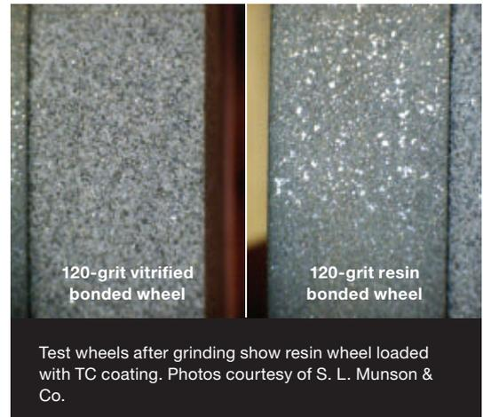
Test wheels after grinding show resin wheel loaded with TC coating. Photos courtesy of S. L. Munson & Co.
